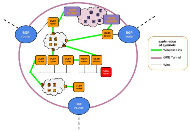
For what concerns the batman-adv nodes, as for the stub area, they do not have any knowledge about the L3 routing issue, therefore they will continue to use as default gateway the edge router assigned by the DHCP protocol.
