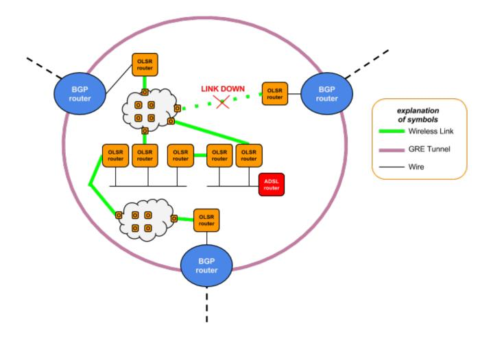
As we see in the figure, we want to handle the scenario in which the BGP router loses its connectivity to its OLSR 2-hop neighbor because the wireless link is down. In this case we need the BGP router to stop announcing upstream the public IPv4 and IPv6 routes of Ninux.
