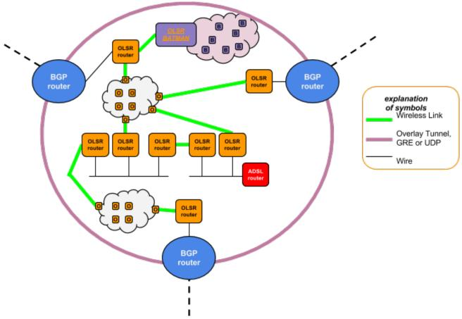
As we see in the figure there will be an edge router between the two domains that speaks both the OLSR and the B.A.T.M.A.N.-Advanced routing protocol. This edge router will announce all the IP addresses used in the batman-adv network with an HNA setting.
